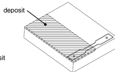
Figure2b – Tension Test Specimen
