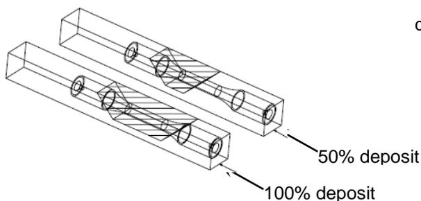
Figure2a – Fatigue Test Specimen
